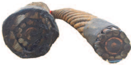
Figure 9: The optical fibre submarine cable of BT-TE-1 on the left and the 1947 Eire P&T submarine cable on the right.
