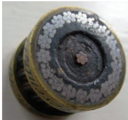
Figure 3: An example of the deep-sea section of 1857-58 trans-Atlantic submarine cable ( www.atlantic-cable.com ).
